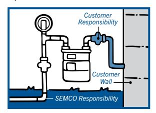
All equipment from the underground piping up to and including your gas meter, as indicated in the diagram, is SEMCO property and is serviced and maintained only by SEMCO Service Technicians or contractors. Customer-owned gas lines and connections between the outlet of the meter and your home, as indicated in the diagram, are the responsibility of the homeowner and should be serviced by a qualified plumber or heating and cooling specialist.
